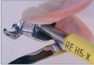
The spring pin is threaded in and out with the RE H 5 tool.
